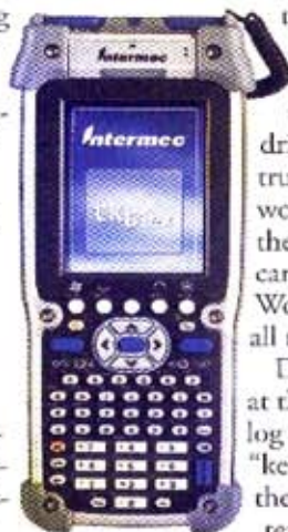
Intermec's CK61ex is a Windows Mobile-based handheld computer with integrated imaging technology for scanning barcodes.
